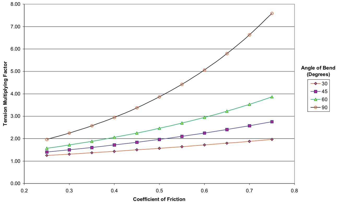
As indicated, the greater the angle of bend, the higher the tension multiplying factor is at a certain coefficient of friction. Assume that 3 cables are being pulled around a 90° bend with a 0.4 coefficient of friction. If there was 1000 lbs. of tension coming into that bend, there would be 2950 lbs. of tension coming out of the bend.
