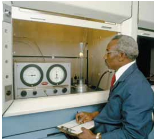
An oxygen index test being conducted in Okonite's Materials Laboratory. This test, in conjunction with other evaluation data, enables the proper selection of insulating/jacketing materials for use in areas where a potential fire risk exists.
