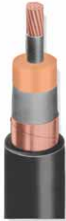
1/C 5/8kV through 35kV Okoguard (EPR) Insulation, shielded, rated MV-105. Okoseal or Okolon jacket available. CT rating also available.
