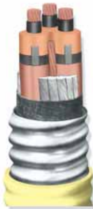
3/C 5/8kV through 35kV CLX Okoguard (EPR) Insulation, shielded, rated MV-105, MC-HL for CT Use, Overall Okoseal jacket.
