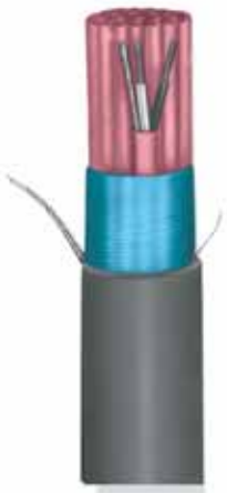
Instrumentation Type SP-OS, Okoseal jacket. 300V PLTC/ITC 600V TC
