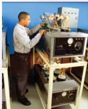
Preparing small wire for long term water immersion testing.
