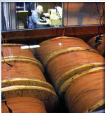
Water tank testing of railroad signal cable.
