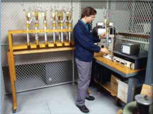
Model cables under test to determine DC characteristics of fluid impregnated paper/polypropylene paper laminate.
