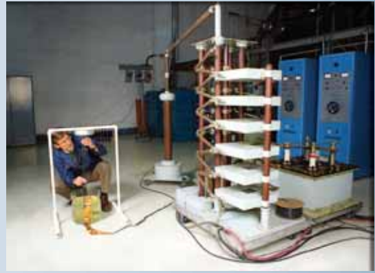
Impulse testing of small wire.
