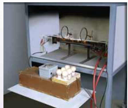
IEC 60331 Circuit Integrity test on Okotherm CIC cable.
