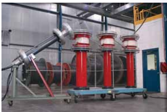
Performing AC voltage widthband test on 69kV Okoguard insulated cable utilizing de-ionized water terminations.
