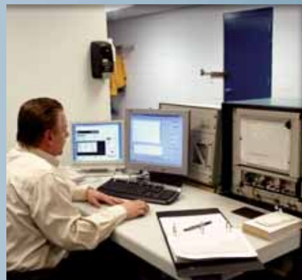
Control console for high voltage AC, DC and partial discharge testing.
