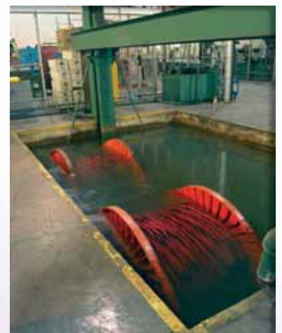
Tank testing of multiple non-shielded cable reels.
