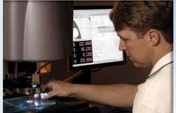
Dimensional check of a cable cross-section using a computer controlled optical comparator.
