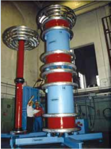
Okonite Research Engineers inspect the 600kV series resonant AC transformer.
