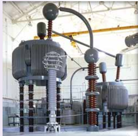
800kV series resonant AC transformer.
