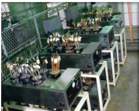
Okoguard and Okonite EPR insulations undergoing long term wet electric stability tests at temperatures from 25C to 90C.
