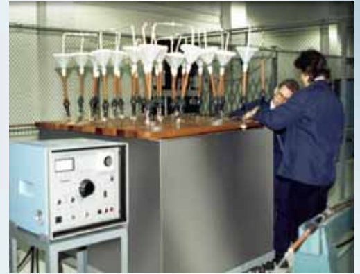
Typical ACLT test tank.
