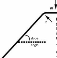
Example: Assume a 1000 Cu kcmil Okoguard-Okoseal Type MV-105 15kV power cable (115-23-3244) with and approximate net weight of 4220 lbs/1000ft or 4.22 lbs/ft. and 1.86" OD (Minimum Bending Radius = 22") is installed on a 30° slope having a 100' length. For this example, we assume a 0.4 coefficient of friction.
