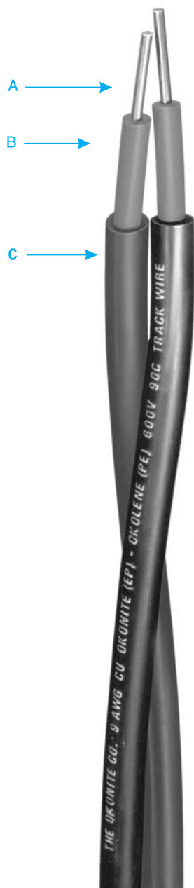
A Solid Uncoated Copper Conductors B Insulation - Okonite-Sizes #9 AWG and #8 AWG-5/64", #6 AWG-6/64" C Jacket-Okolene, Color Coded; 1-Black, 1-Red
