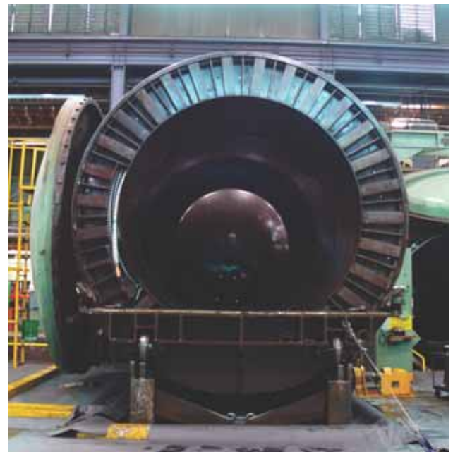
Horizontal Tank capable of impregnating up to 345 kv HPFF cables in lengths of 6,500 to 12,000 feet on 188" diameter reel.
