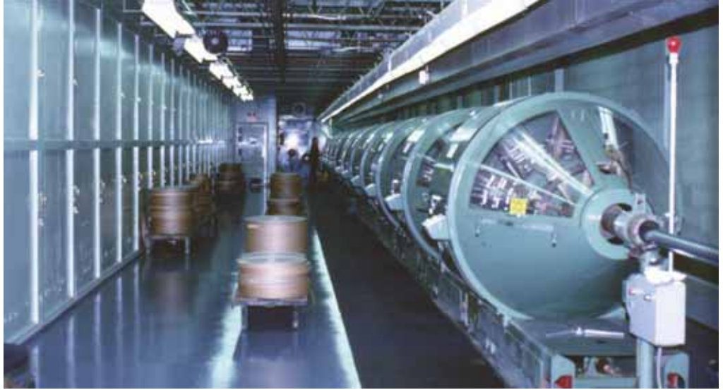
One of two EHV voltage taping head machines.
