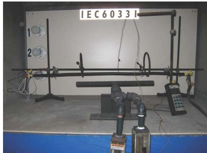
Cable setup prior to flame test.
