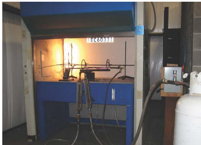
Energized cable undergoing flame test.
