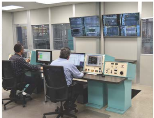
Test department includes test pens for efficient operations and material handling. Equipped for AC or DC testing, dry and water tank testing of cables.
