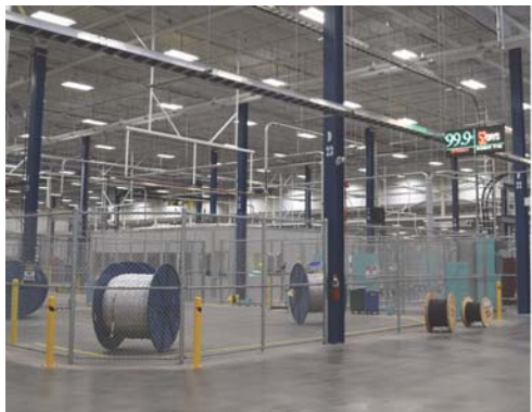
Test department includes test pens for efficient operations and material handling. Equipped for AC or DC testing, dry and water tank testing of cables.
