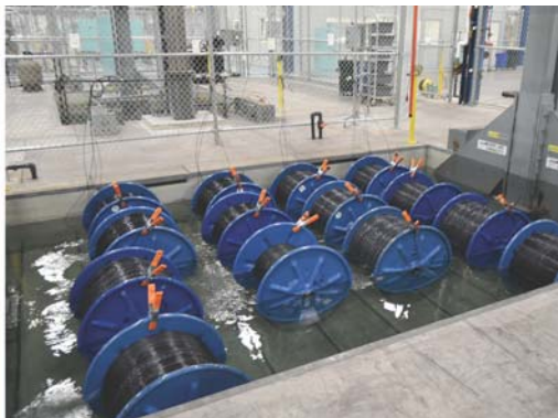
Test department includes test pens for efficient operations and material handling. Equipped for AC or DC testing, dry and water tank testing of cables.
