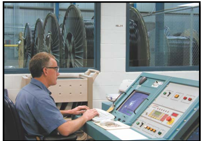
Corona test on single conductor prior to cabling
