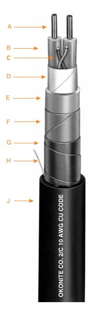
A Uncoated, Solid Copper Conductors B Insulation—Okolene C Communication Pair D Polyester Tape E Okolene Belt F Polyester Tape G 5 mil Copper Shield H Pull Cord
