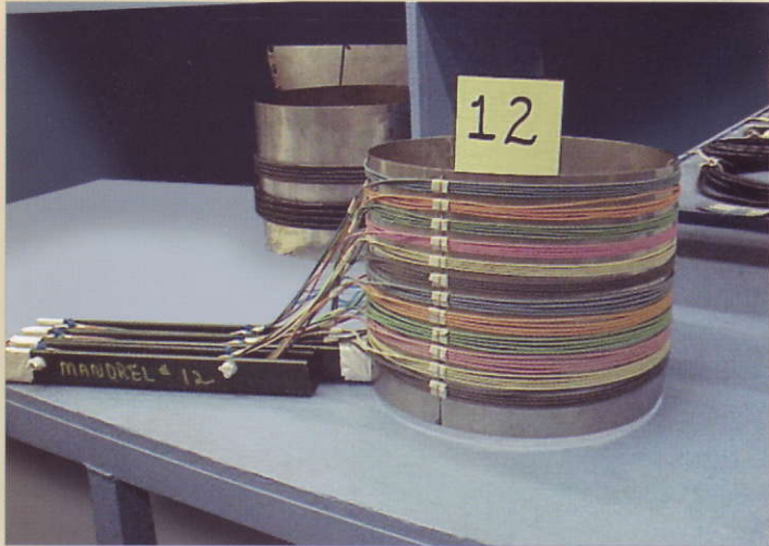
Insulated conductors on prepared mandrels for LOCA simulation
