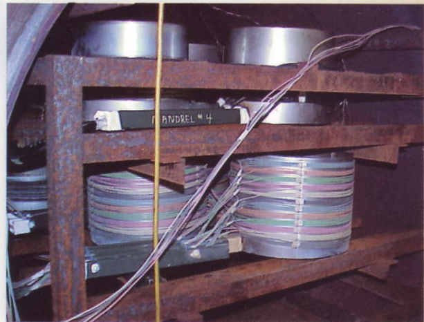
Loading mandrels in LOCA test vessel awaiting commencement of test
