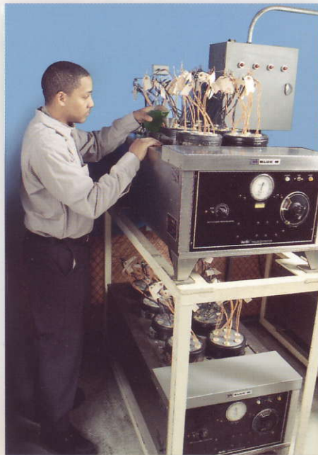
Long term electrical moisture stability testing of insulation compounds.
