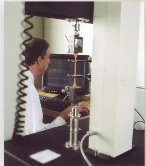
Physical testing of installation and jackets for tensile strength and ultimate elongation
